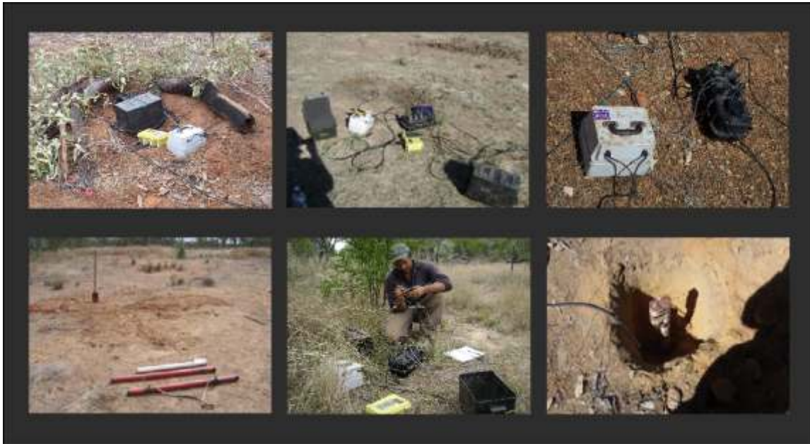
Various images showing layout of field equipment including recording boxes, cables, electrode and buried magnetometer sites.
