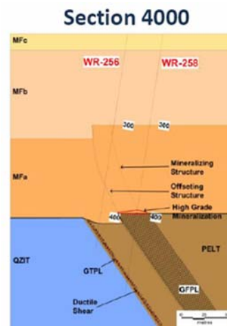
Simplified geology from Wheeler River showing geologic model of fault-associated Uranium at Unconformity surface.
